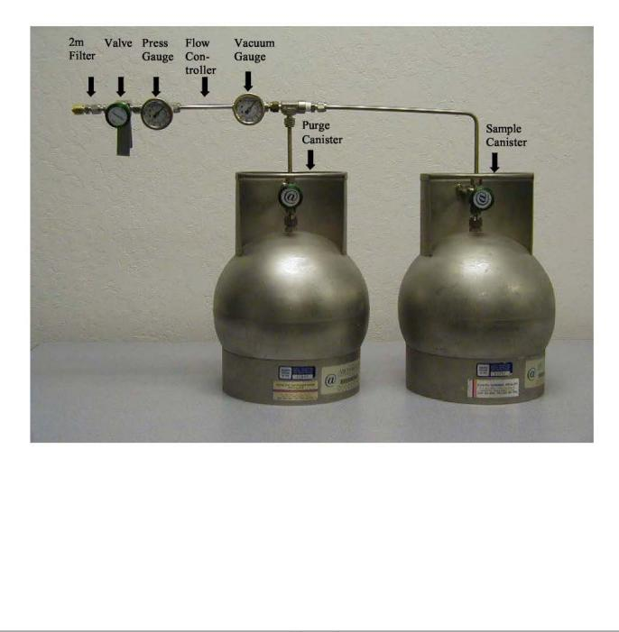
Figure 3 Typical Soil Gas Sample Collection Manifold Xtra Oil Company 1701 Park Street Alameda, California
