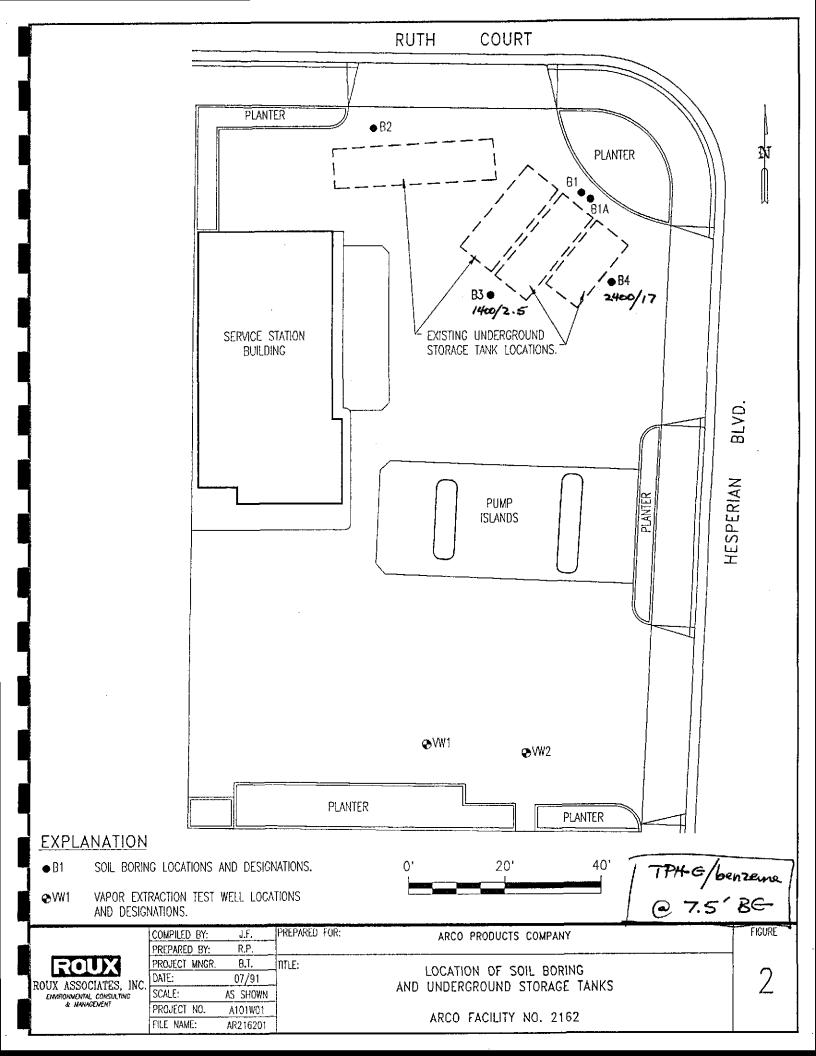
to a planned replacement of USTs. The field investigation involved the drilling of seven soil borings, collection of undisturbed soil samples and installation of two vapor extraction test wells. The wells will be used to evaluate the feasibility of using vapor extraction techniques at the Site (Figure 2).
