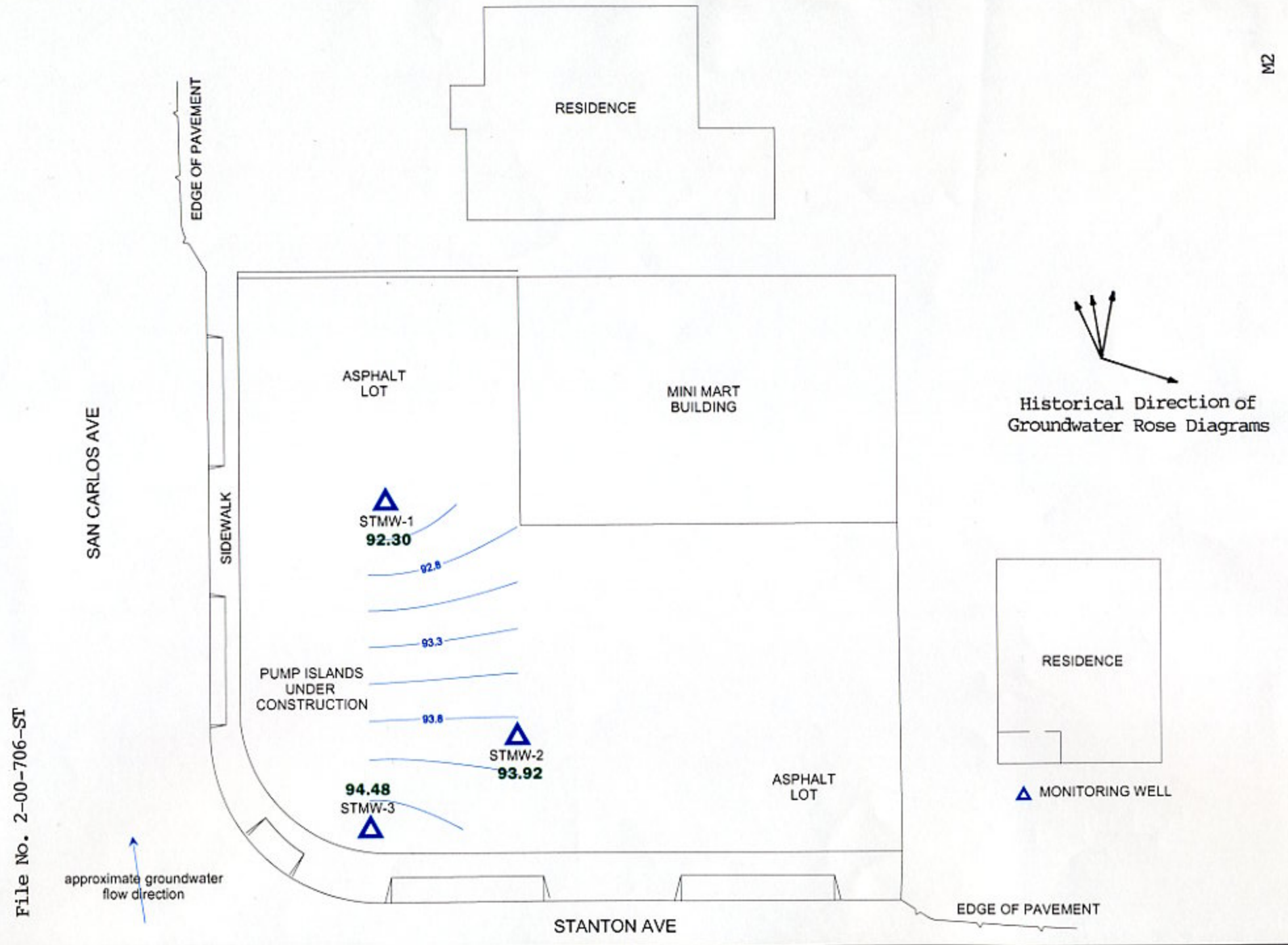
Figure 2: Groundwater elevation contour in feet. March 24, 2005.
