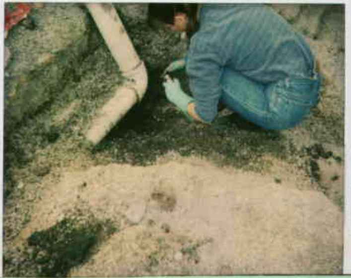
7/6/93 - Photo taken by 2215117976-B Ron Owsatz at Bansal shell, 2120 Montana Ave, Oak. Shown is Allison Watts taking soil sample at end of old piping where some soil cont. was observed. (R)
