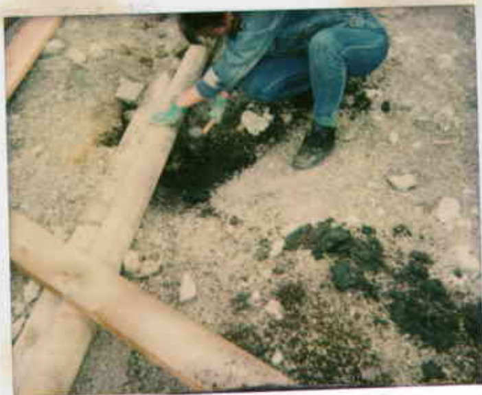
7/6/93 - Photo taken by Ron Cuccare at Banzal Shell, 2120 Hartana Ave, Oak. Shown is Allison Watts taking soil sample under middle of old piping where some soil cont. was observed. ②
