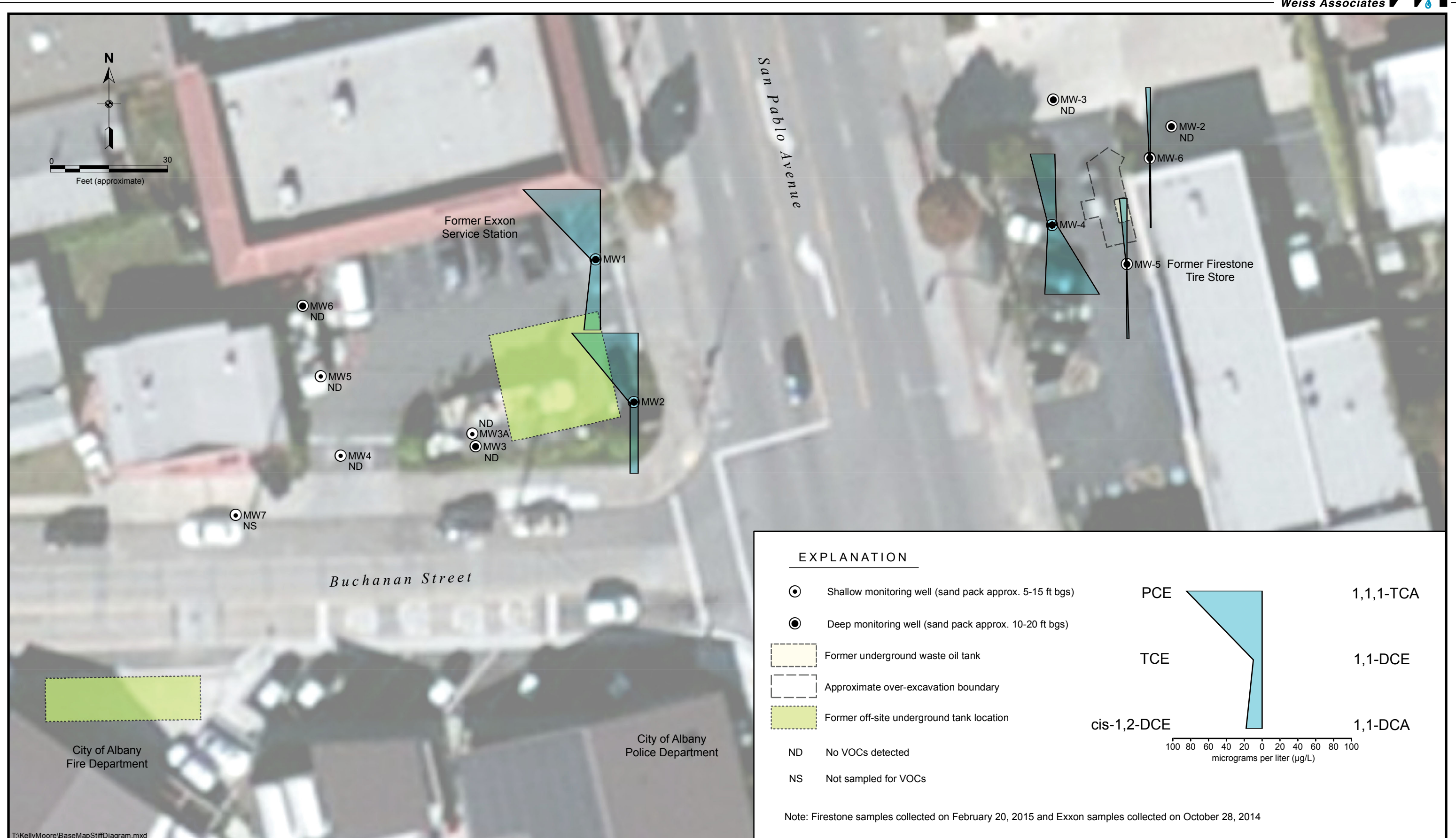
Figure 6. Modified Stiff Diagrams Depicting VOC Concentrations in Groundwater, Former Firestone Tire Store #3655, 969 San Pablo Avenue, Albany, California
