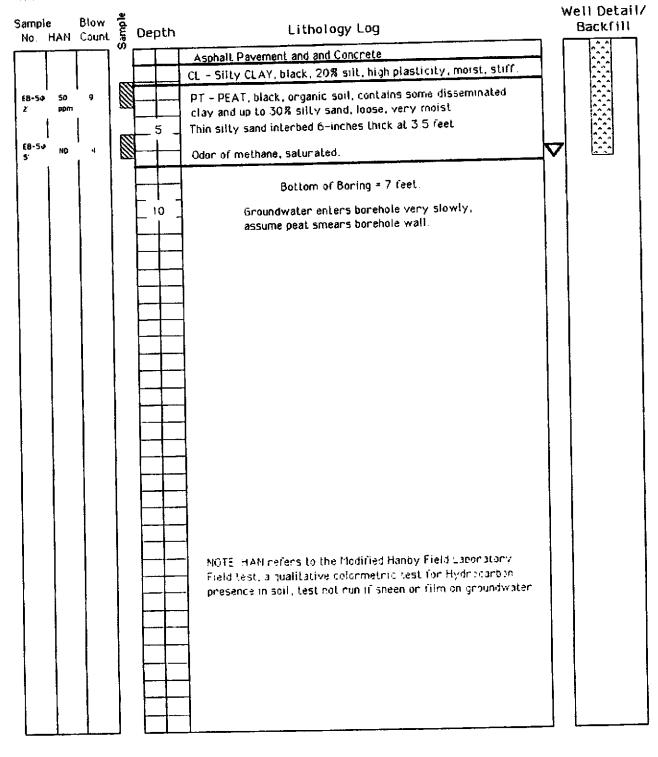
Project No. 9407 Boring/Well No. EB-7 Client: DiSalvo Trucking Date Drilled: April 7, 1994 Location: 4919 Tidewater, Oakland, CA Logged by: EL Drilling Method: Hollowstem Auger Permit: N/R Water Levels: 1st Enc: 3.5' Static: no measurement Exploratory Boring Log Borehole Completion Well Installed: NO
