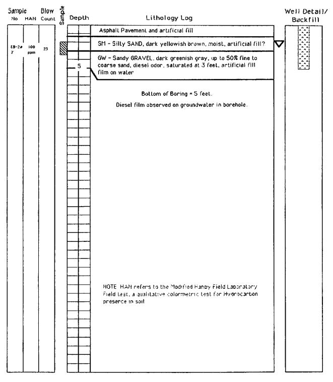
Project No. 9407 Boring/Well No. EB-3 Client: DiSalvo Trucking Date Drilled: April 7, 1994 Location: 4919 Tidewater, Oakland, CA Logged by: EL Drilling Method: Hollowstem Auger Permit: N/R Water Levels: 1st Enc: 3.2' Static: no measurement Exploratory Boring Log Borehole Completion Well Installed: NO
