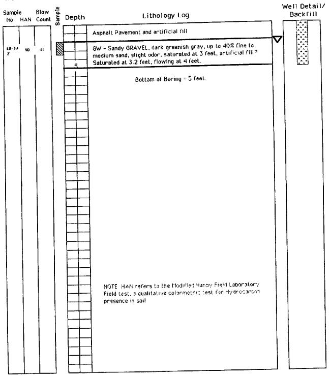
Project No. 9407 Boring/Well No. EB-4 Client: DiSalvo Trucking Date Drilled: April 7, 1994 Location: 4919 Tidewater, Oakland, CA Logged by: EL Drilling Method: Hollowstem Auger Permit: N/R Water Levels: 1st Enc: 2.8' Static: no measurement Exploratory Boring Log Borehole Completion Well Installed: NO
