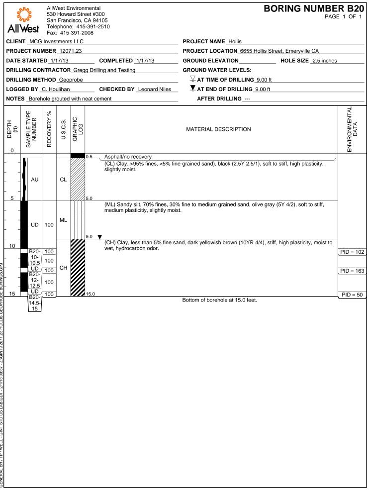
GENERAL BH / TP / WELL - GINT STD US LAB.GDT - 2/1/13 09:37 - Z:\GINT/12071.23 HOLLIS GEOPROBE BORINGS.GP.
