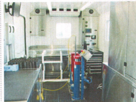
Stainless steel interiors on all CPT rigs provide laboratory space for collecting environmental samples and decontaminating equipment.
