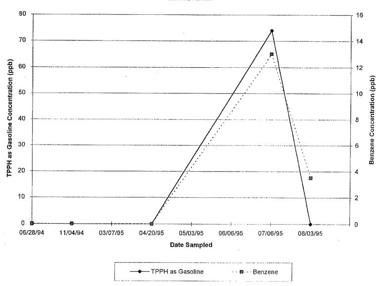
Figure D-3 Soil Vapor Extraction System Mass Removal Trend
