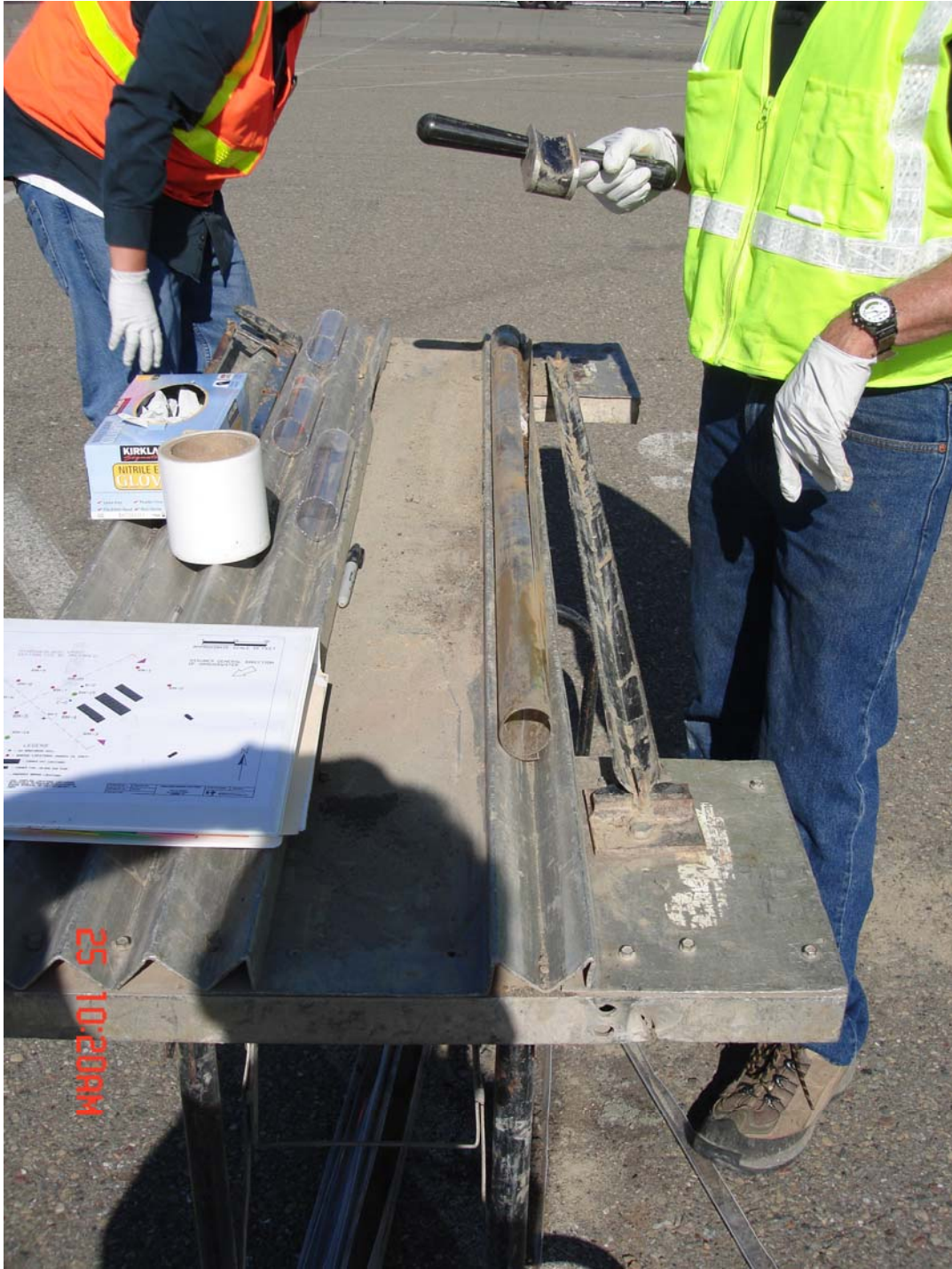
Photo #6 - The geologist visually inspecting and describing soil samples according to the Unified Soil Classification System.
