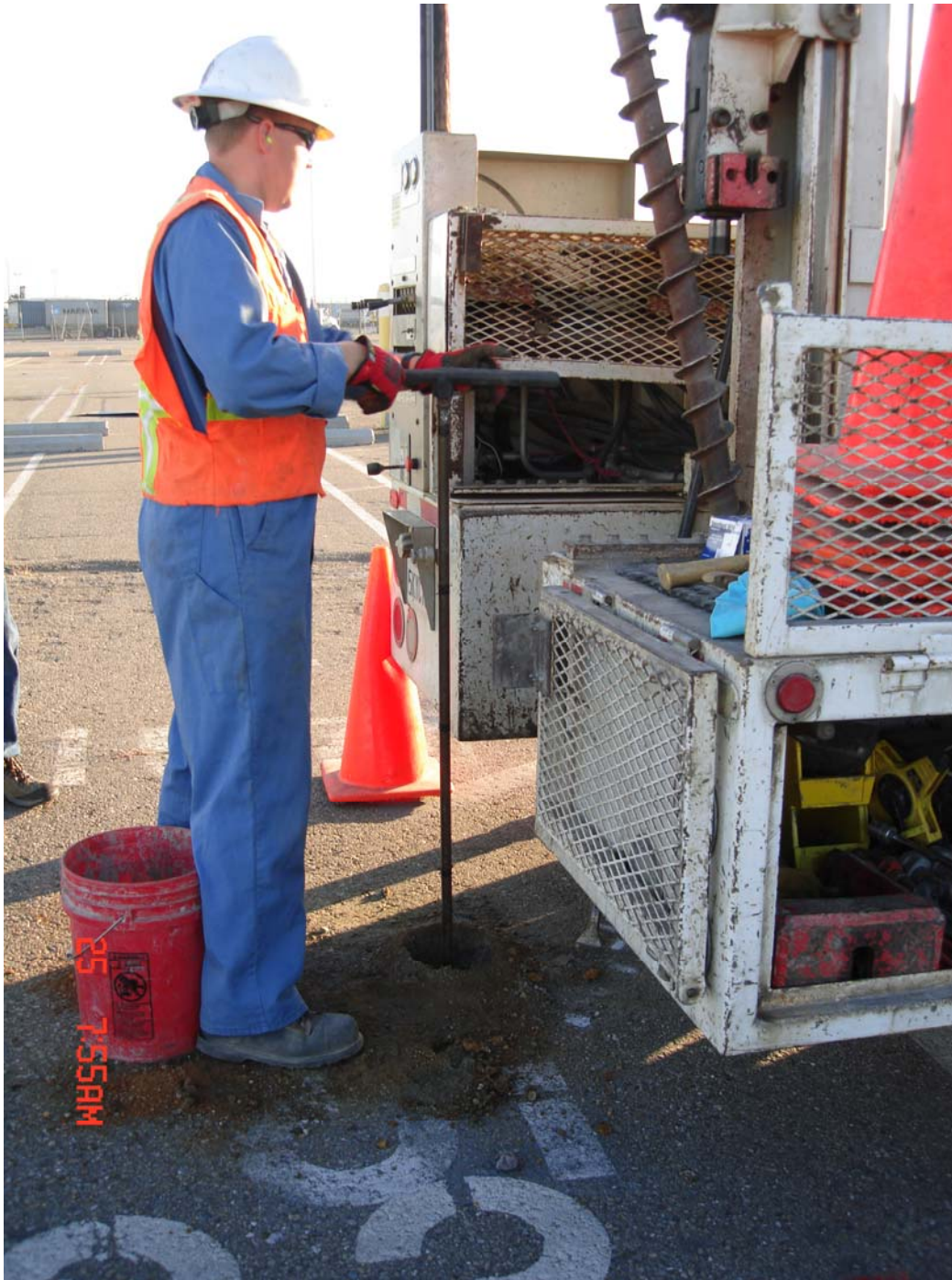
Photo #5 - Hand augering boreholes to a depth of 5 ft before employing the "direct push" method.
