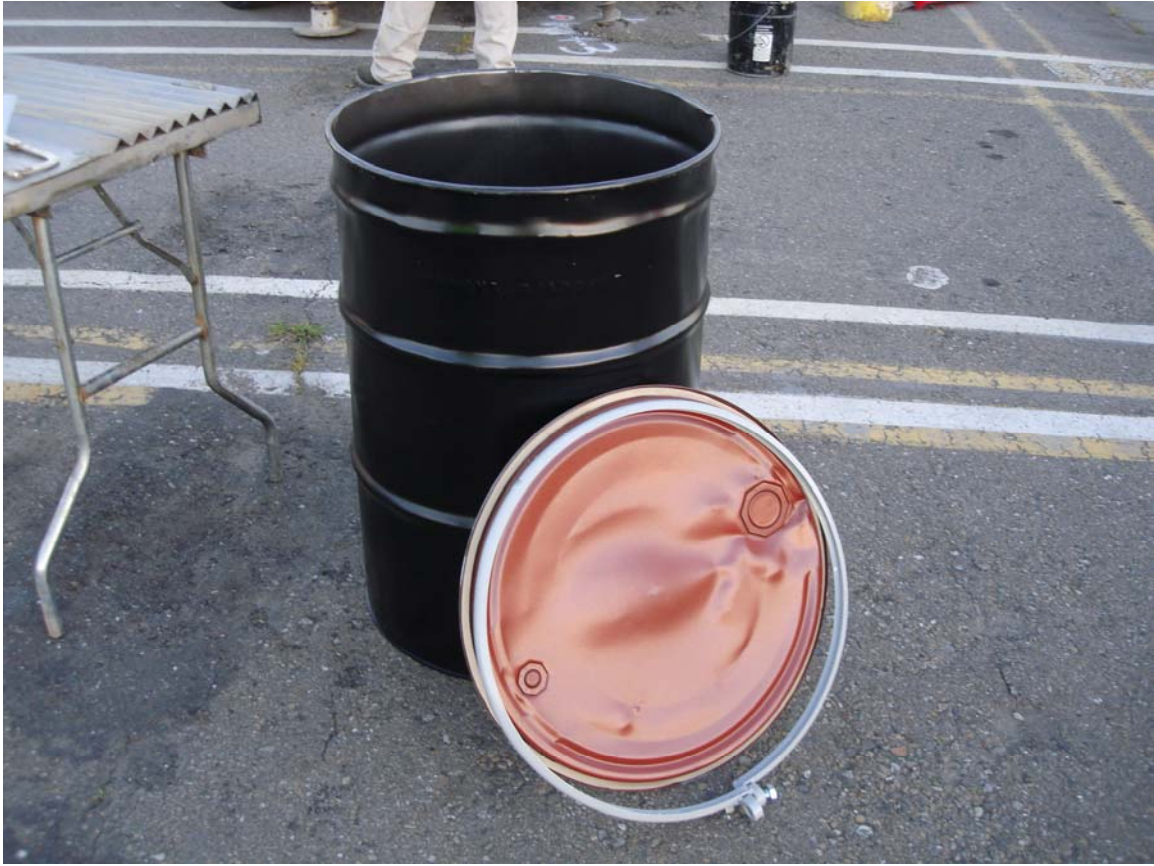
Photo #11 (3/15/07) - 55-gallon drum used for storage of IDW
