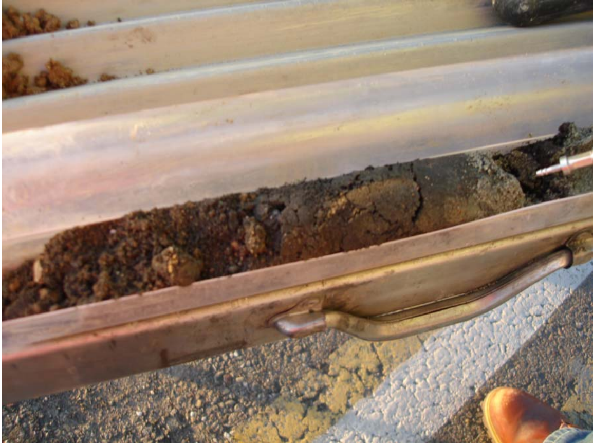
Photo #6 (3/15/07) - Obtaining PID readings for initial 5-9 ft soil sample from RM-3
