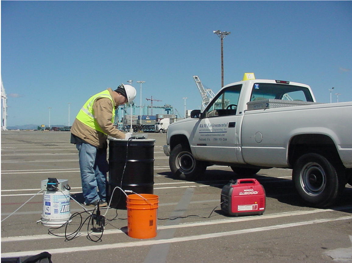
Photo #13 (4/12/2007) – Pumping 3 casing volumes of water before collecting groundwater samples from well MW-1
