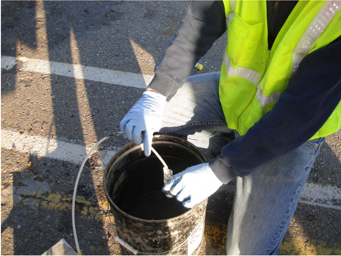
Photo #9 (3/15/07) - Collecting groundwater sample in 40-ml VOAs preserved with HCL
