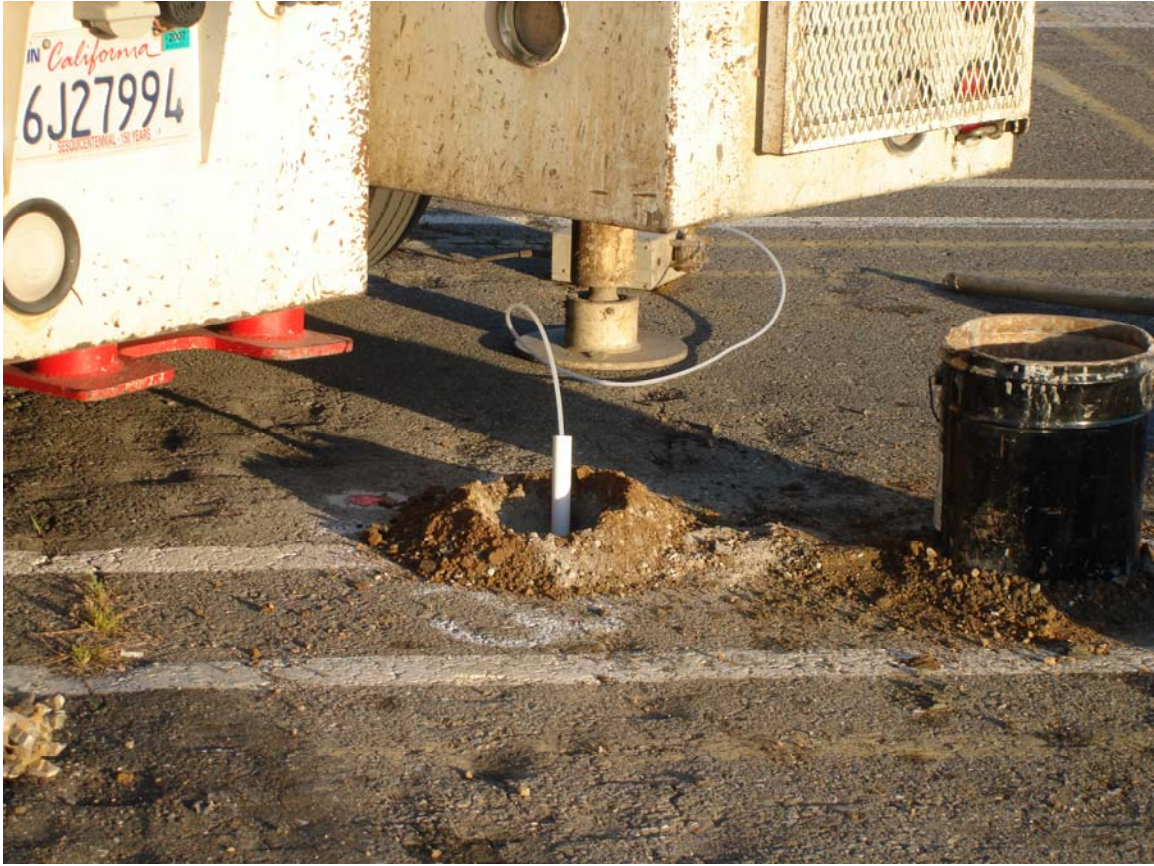
Photo #8 (3/15/07) - Purging 1-2 gallons from RM-3 using a peristaltic pump, prior to collection of groundwater sample
