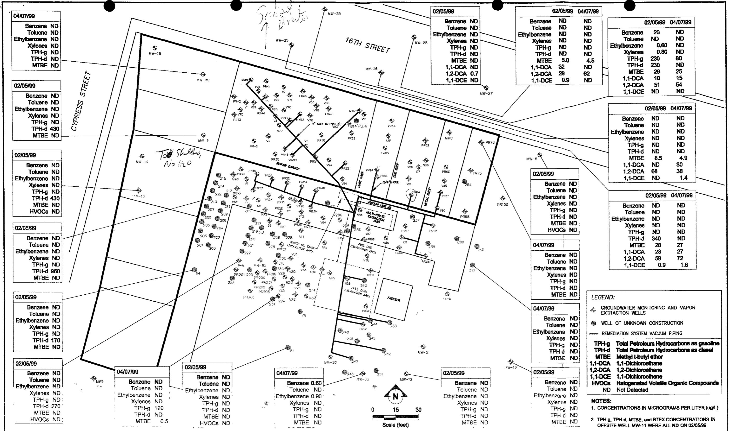
SITE PLAN SHOWING GROUNDWATER ANALYTICAL RESULTS, FEBRUARY AND APRIL 1999 NESTLE OAKLAND FACILITY 1310 14th STREET, OAKLAND, CALIFORNIA
