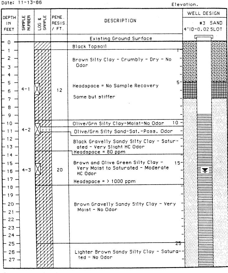
Figure 3A - Test Boring Log No. 1 - Monitoring Well No. MW-4
