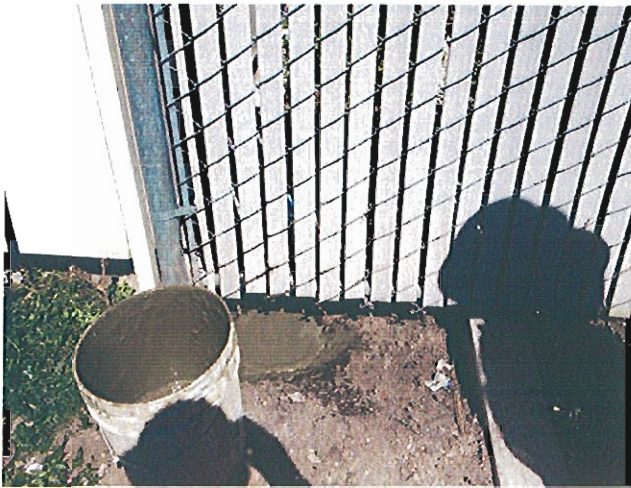
Photo 7: Over-fill of well MW-5
